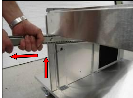
Figure 26b: Lift and pull forward
