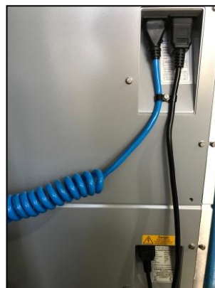
Figure 4a: Mains connection point
