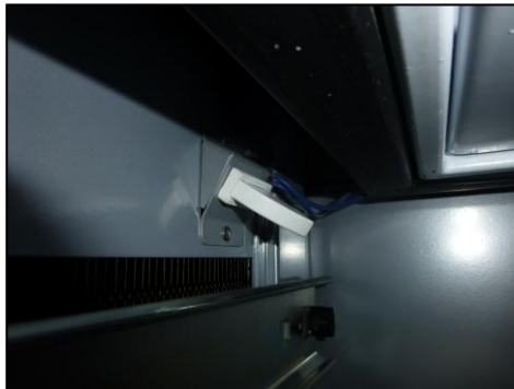
Figure 18c: Drawer switch mounted in the chassis
