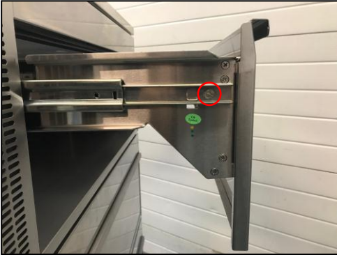
Figure 25a: Remove support cradle retaining screws
