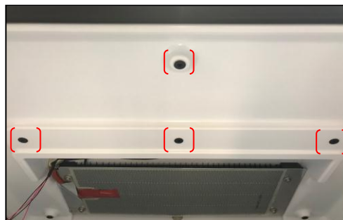
Figure 19c: Rubber fastenings in situ
