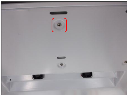
Figure 19a: Diffuser screws in situ
