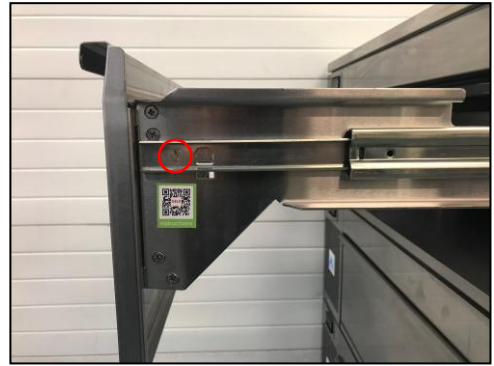
Figure 25a: Remove support cradle retaining screws
