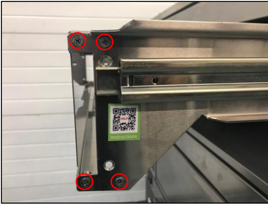
Figure 15: Removing the eight M5x 8 ST/ST screws
